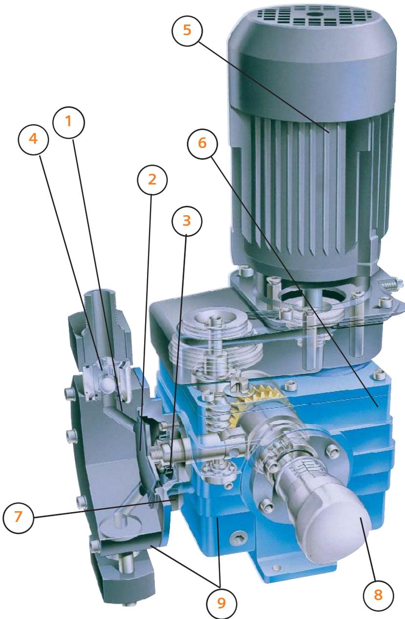
The Encore® 700 diaphragm metering pump is available in two compact drive arrangements: direct drive or pulley drive for an additional 4:1 range ability on stroke frequency with a standard induction motor. When the pulley drive arrangement is combined with a DC variable speed motor, total operating turndown can be as high as 800:1.
