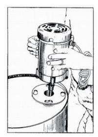
**Step 2**Mount Motor/Shaft
