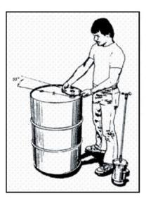
**Step 1**Install mounting flange in 2" (5.1 mm) bung opening. Tighten by hand until flange is firmly seated.
